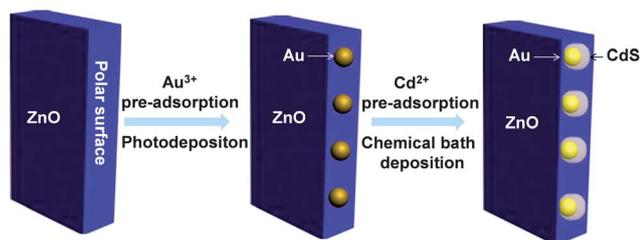
**Fig. 1** Schematic of the preparation route of a CdS/Au/ZnO heterostructure through a two-step self-assembly process induced by the surface polar charges of ZnO.
