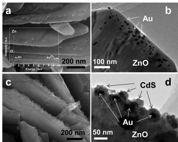
**Fig. 3** (a and b) SEM and TEM images of Au/ZnO; (c and d) SEM and TEM images of the CdS/Au/ZnO heterostructures. The inset in (a) is the EDS spectrum of Au/ZnO.
