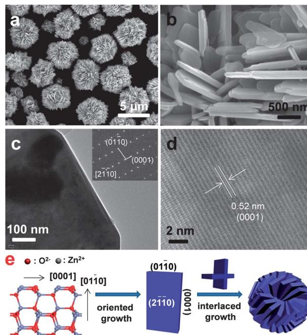
**Fig. 2** (a and b) Low-magnification and high-magnification SEM images of flower-like spheres of ZnO crystals; (c and d) TEM and high-resolution TEM images of a single ZnO nanosheet. The inset in (c) is a corresponding SAED pattern; (e) schematic of the formation process of a flower-like ZnO sphere.
