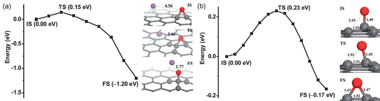
**Fig. 4** (a) Transformation intermediate states during the lithiation of  $\text{C}=\text{O}$ . (b) Transformation intermediate states from delithiated  $-\text{O}-\text{C}$  to  $\text{Li}-\text{O}-\text{C}$  (epoxide). Bond length and distance between atoms are in units of Å. Lithium: purple ball. Oxygen: red ball. Carbon: grey ball. X-Axis represents the reaction coordinate: IS: initial state, TS: transition state, and FS: final state.
