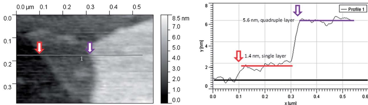
**Fig. 1** (Left) AFM topographical image of stacked GO nanosheets deposited on a Si substrate. (Right) Cross-section profile at different positions along the line in the left panel, revealing mono- and quadruple layer structures (generated by Gwyddion freeware software).
