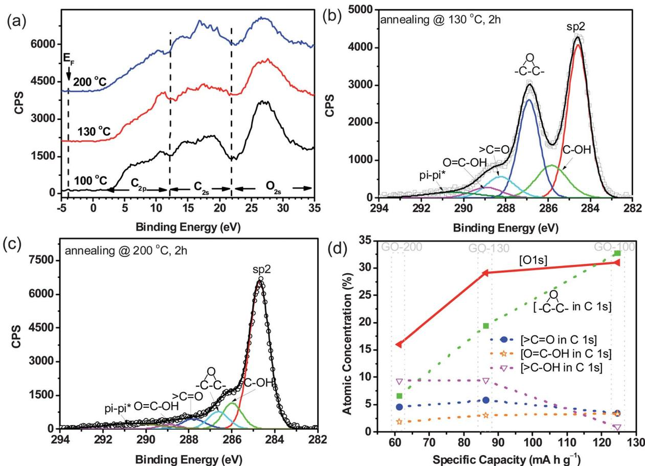
**Fig. 3** (a) VB spectra of GO cathodes annealed at 100 °C, 130 °C and 200 °C for 2 hours. XPS C 1s spectra of (b) GO-130 and (c) GO-200 cathodes. (d) The FTIR spectra of the GO-100, GO-130 and GO-200 cathodes. (d) Relationship between discharge capacity @ 0.5 A g<sup>-1</sup> and the atomic concentrations of O 1s and oxygen functional groups in C 1s (epoxide (◡◡), hydroxyl (>C-OH), carbonyl (>C=O) and carboxyl (O=C-OH)).
